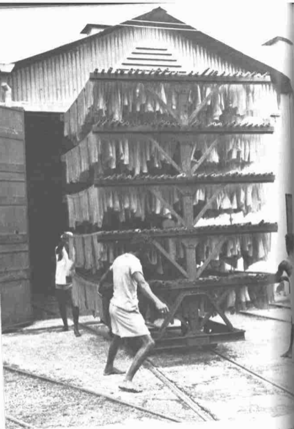
After it has been chopped into sheets the rubber is hung on a drying rack, and this is then pushed into a drying room. After that it is smoked for about five days.
